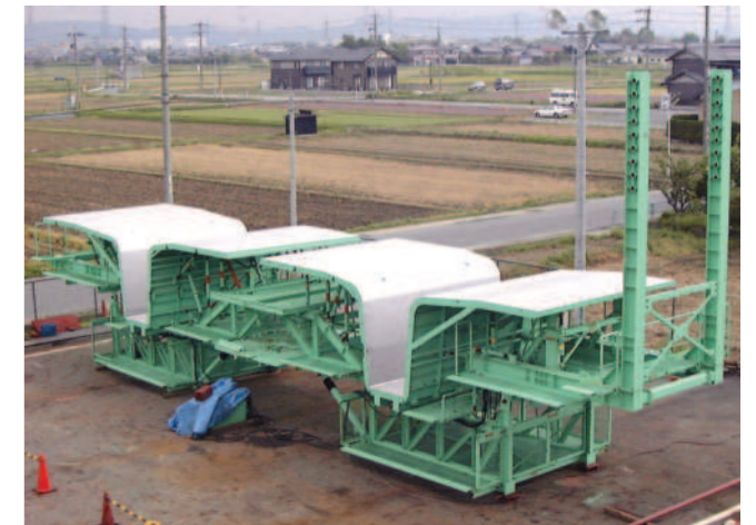
MOVING STEEL RIG MADE OF STAINLESS STEEL
