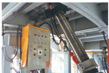
← 油圧開閉式伸縮打設孔・ピストン型枠装置 Oil Hydraulic Open/Close Type Elastic Concrete Nozzle & Formwork Piston System
