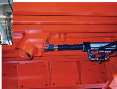
← 油圧開閉式伸縮打設孔・ピストン型枠装置 Oil Hydraulic Open/Close Type Elastic Concrete Nozzle & Formwork Piston System
