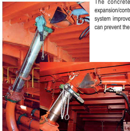
↑ 油圧開閉式伸縮打設孔 Oil Hydraulic Open/Close Type Elastic Concrete Nozzle
